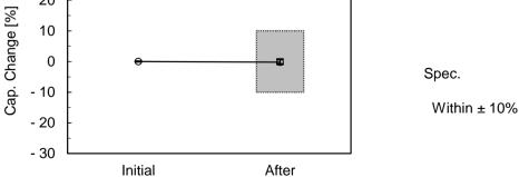
(Dielectric Strength) AC2600V(r.m.s.),60 s and DC3225V,60 s Dielectric Strength (Between lead wires) : No failure Dielectric Strength (Body Insulation) : No failure Insulation Resistance (I.R.) :  $1000M\Omega$  min. Appearance : No marked defect
